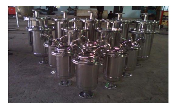
The Candle Filters are installed for clarification and recovery applications from liquids with low solids content. They are an ideal replacement for manual pressure filters and other equipment where solids, solvents and hazardous materials are being handled.
